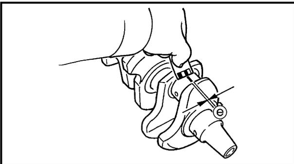
c. Put a piece of Plastigauge® ① on the crankshaft pin.
