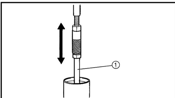
12. After filling the front fork leg, slowly stroke the damper rod ① up and down (at least ten times) to distribute the fork oil.
