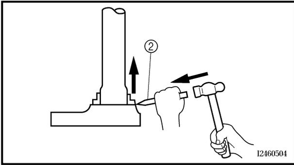
b. Remove the bearing race from the lower bracket with a floor chisel ② and hammer.
