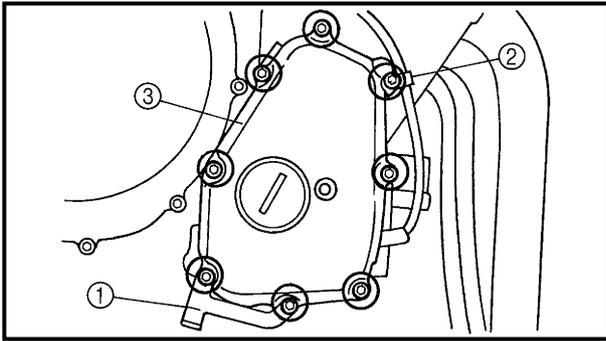
**REMOVING THE PICKUP COIL ROTOR**
