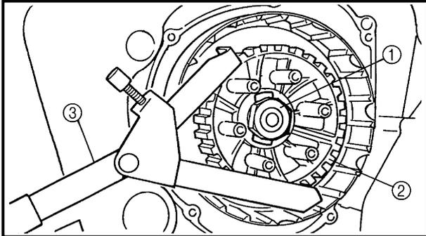
2. Straighten the lock washer tab.
