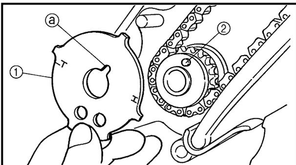
**INSTALLING THE PICKUP COIL ROTOR**
