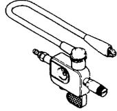
A technical drawing of an ignition checker tool. It consists of a long, thin metal rod with a hook-like end, attached to a central body with various adjustment points and a threaded end. |
