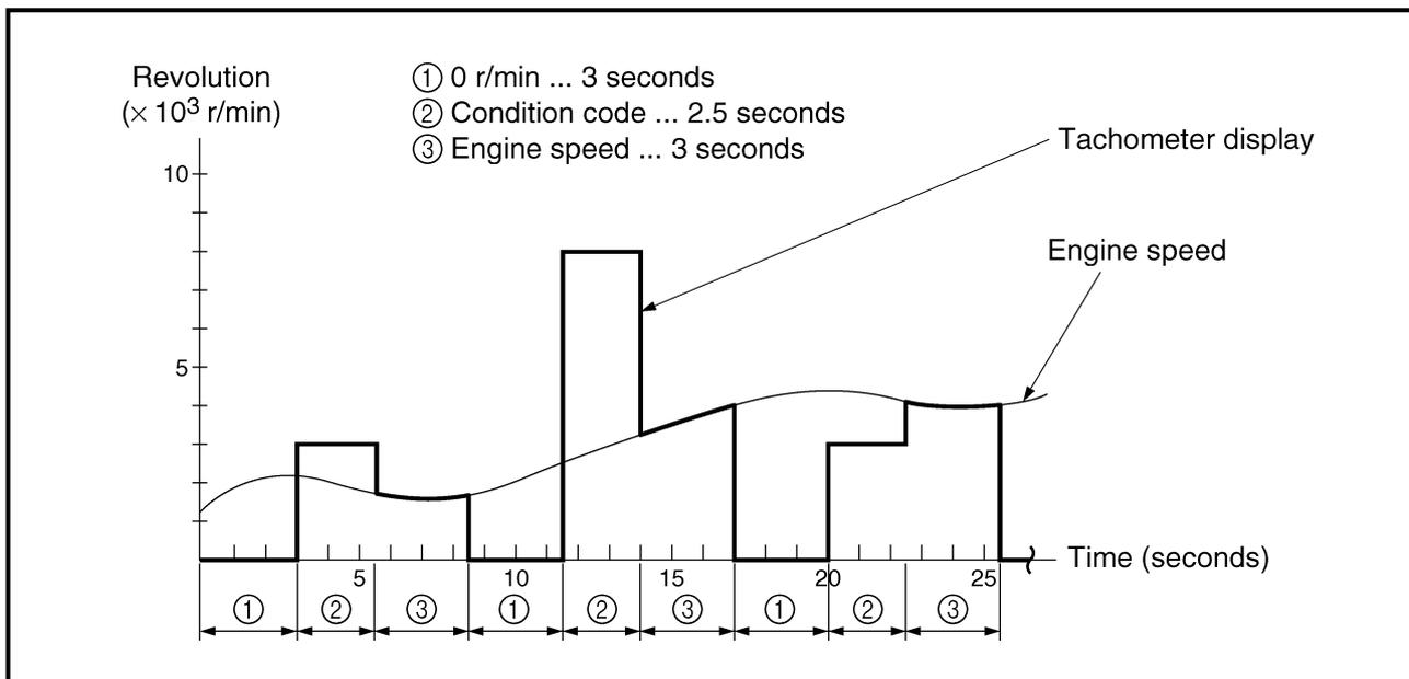
When more than one item is being monitored, the tachometer needle displays the condition codes in ascending order, cycling through the sequence repeatedly.
