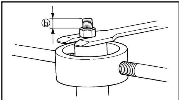
c. Install the rod puller and adapter onto the damper rod.
