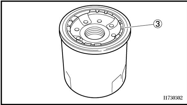
b. Lubricate the O-ring ③ of the new oil filter cartridge with a thin coat of engine oil.
