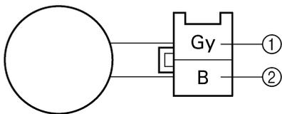
• Measure the pickup coil resistance.
